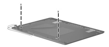
Where used: 2 screws that secure the display hinge covers to the display enclosure
